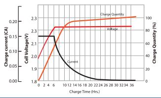
Temperature: 27 deg C Discharge: 100% C10 rate Recharge: 2.23 vpc 0.15C Amps
