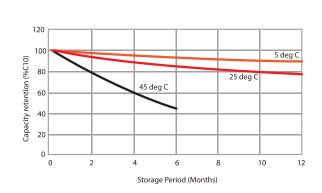
Supplementary charge is recommended before capacity retention ratio drops less than 80%.
